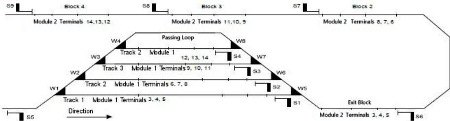
So that none, or a minimum number of track connections are unused, different operating modes can be combined in a module under certain circumstances. This cannot be achieved when using the simple key programming and must be done by using LocoNet programming (see Chap. 1 "General").
