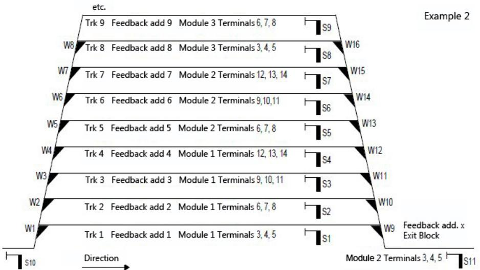
If a station with an automatic Entry and Departure has (Example 2) more then 6 tracks then additional modules for more tracks can be installed.
