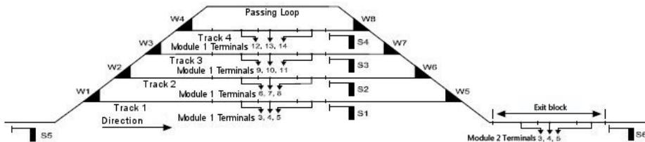
For an automatic station control two modules are installed. As long as the station entry is not switched manually the entry turnouts to the passing loop are controlled by a second Universal Control which controls the station entry and first 4 tracks.
