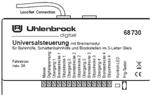
The two LocoNet sockets on the Universal Control are identical and can be used for connecting the center or further LocoNet devices.
