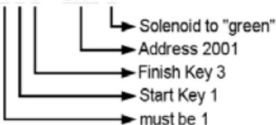
Start Key 2 and Finish Key 1 switches solenoid address 2002 red and thus Route 3 from Group 1 in the Intellibox.
