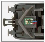
Connection of the LISSY Mini transmission module to the decoder is described in the respective decoder manual.
