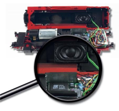
For the Ho range we offer various loud speakers with resonance shells. The important point when selecting a loud speaker is: the larger the speaker the fuller the sound.
