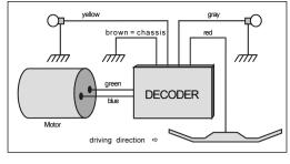
connection must be kept. Should the directional lighting come on wrong, change the green and blue leads on the motor. Connect both outputs with each other if you wish them to work direction-independently.
