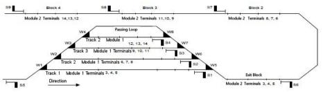
So that none, or a minimum number of track connections are unused, different operating modes can be combined in a module under certain circumstances. This cannot be achieved when using the simple key programming and must be done by using LocoNet programming (see Chap. 1 "General").
