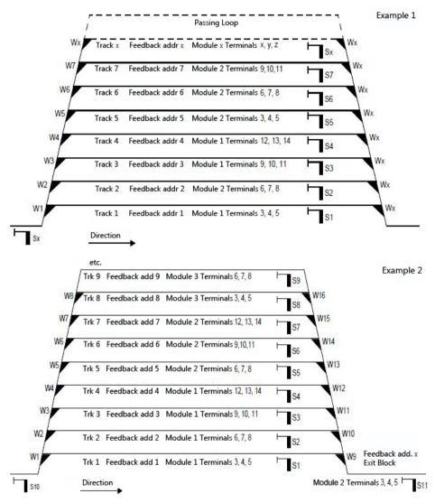
If a station with an automatic Entry and Departure has (Example 2) more then 6 tracks then additional modules for more tracks can be installed.
