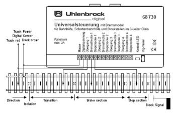
The running section must be long enough so that it can accommodate the longest train. The braking section must be long enough for the train with the longest braking distance. The optional stop section is without power when the brake generator (Signal Halt), so that trains which may slip through are always safely stopped.
