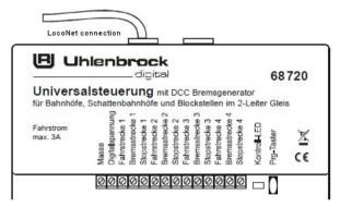
The two LocoNet sockets on the Universal Control are identical and can be used for connecting the center or further LocoNet devices.
