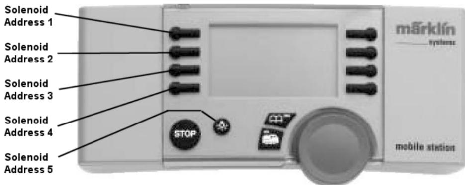
The solenoids can be switched using the special function keys. If the solenoid is in the “round” or “red” state, pressing the key once will switch the solenoid over to “straight” or “green” and vice versa. The solenoid status can not be read on the mobile station.
