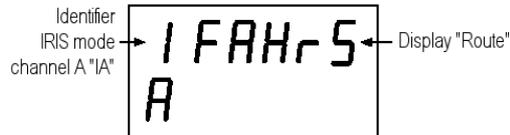
The display shows the route number with a bouncing bar before it. This will continue until the route is fully processed by the Intellibox.
