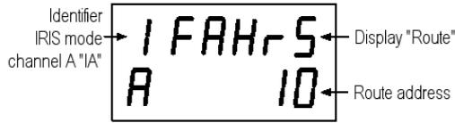
If subsequently, a route number is entered using digit keys on the remote control, then this input can be monitored on the display.
