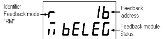
If the address value of the indicator buffer is set to a value between 1 and 2033, the display shows the status of 16 feedback modules. The display begins at the top left with the status of the feedback module whose address is programmed the indicator buffer. The following locations will display the status of the next 15 feedback modules:
