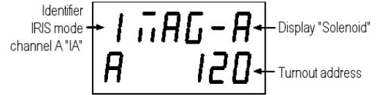
If turnout base address is changed at the remote control, the appropriate inputs can be read from the display.
